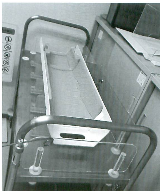
Fig.1 MRI Cradle for newborn baby and infant. This MRI cradle has been made in our hospital. The examination could thus done with safety.
